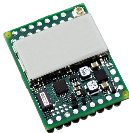
Figure 2 | The MicroGRAM GPS receiver from Rockwell Collins can be used on a small UAV, a tactical radio, and even a rifle site.
